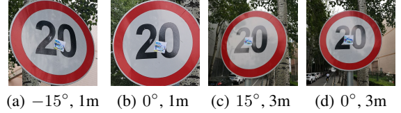
Figure 7: Traffic signs with adversarial patches on them. The photos are taken in the campus of Beihang University with different distances and angles using camera. Traffic signs are respectively classified as “No Entry”, “Slippery Road”, “Speed Limit 60” and “Over-weighted Vehicles Prohibited”.
